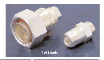
Microlab TA series terminations are low power coaxial loads, which operate from DC to 2.5 or up to 18 GHz depending on the model. Each has been designed with a resistive film terminating element, contained within a carefully matched coaxial housing.
